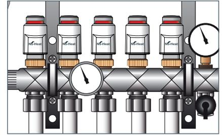
At this stage the blue protection caps can be replaced with actuator heads on each manifold port.
