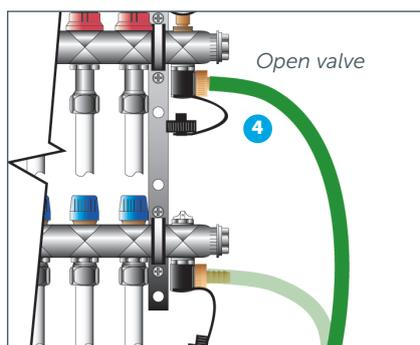
**4** Remove the blanking cap from the filling valve on the flow (upper) manifold. Fit the hose connection nozzle (from the [Tools and Accessories Pack](#)), and connect a suitable hose from the mains water supply. Open the filling valve using the key on the blanking cap.
