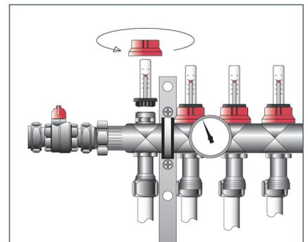
**3** Fully open all the flow adjusters on the supply (top) manifold by lifting and inverting the red locking collar which may then be used to turn the black collar fully anti-clockwise.
