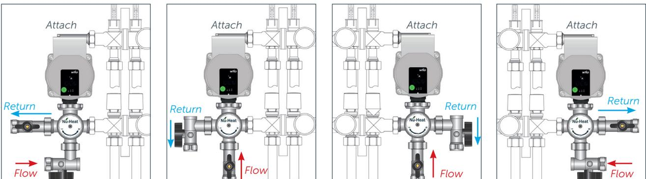
5 Take the elbowed pump connector and attach this to the top of the pump with the free end pointing in the opposite direction to the isolating valves.
