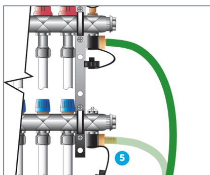
**5** Similarly fix a suitable hose to the drain valve on the return (lower) manifold.
