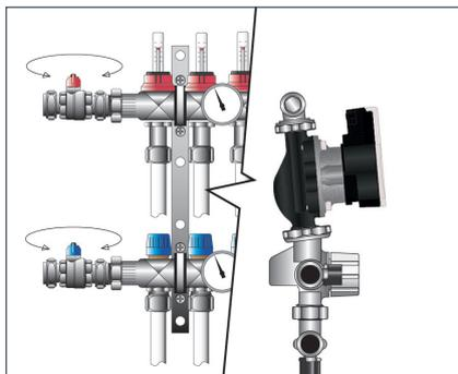
**1** Close the isolating ball valves that are either connected directly to the manifold, or connected just before the Direct Mounted Pump Module.
