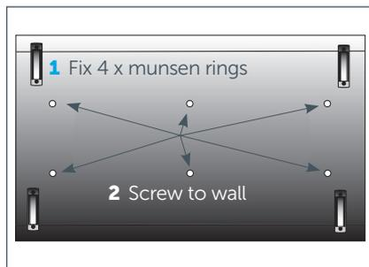
The Remote Mounted Pump & Valve Module should be screwed to the wall using the holes provided in the backplate.
