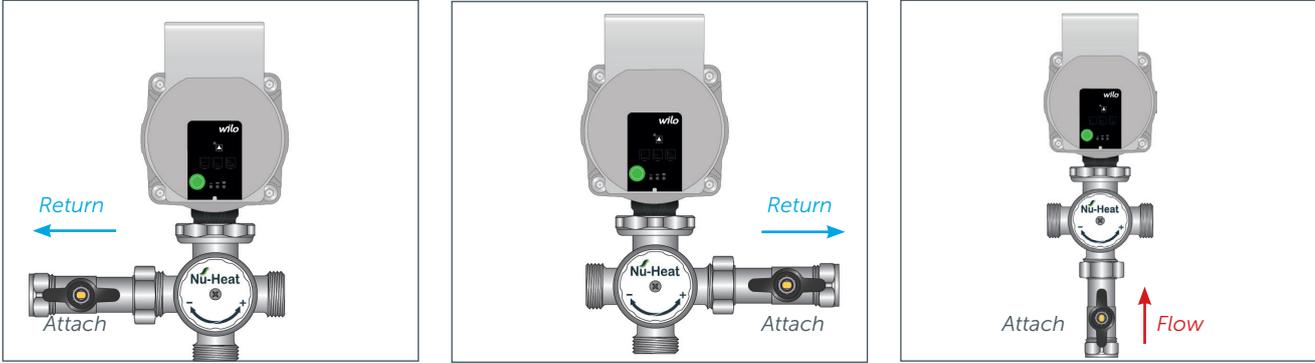
3 Take the straight isolating valve and attach to the left-hand side, right-hand side or bottom of the blending valve as required.
