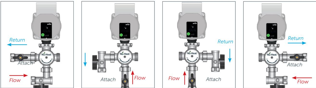
4 Attach the other isolating valve to the bottom of the temperature blending valve using the attached captive nut and rubber washer provided. The two valves must be pointing in the same direction.
