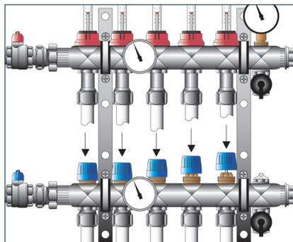
**2** Isolate all zones by screwing down all the blue protection caps hand tight.
