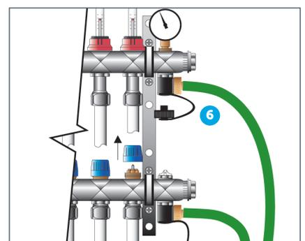
**6** Fully loosen the protection cap from the first zone to be filled.
