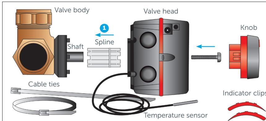
**Note:** Two versions of the red indicator clip are supplied to indicate whether the valve is fully open or fully closed to the boiler flow.
