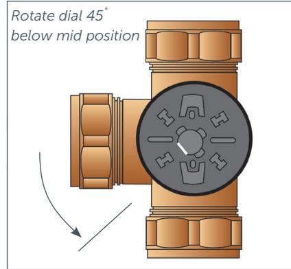
Use the plastic knob provided to turn the valve position such that the flat face with the arrow faces at  $45^\circ$  below the mid position (see diagram). The shaft must be set to the correct position prior to fixing the electric actuator motor.
