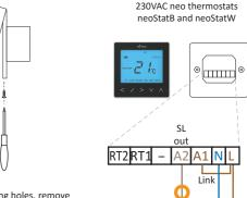
To access fixing holes, remove screw below thermostat body. Pivot front face away from backplate
