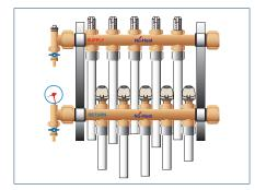
Check that the relevant actuator on the underfloor heating manifold operates correctly. Actuators take approximately three minutes to respond.
