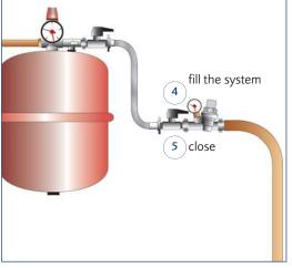
**4.** Fill the system via the boiler filling loop and run water through until the flow from the drain hose is free from air bubbles.
