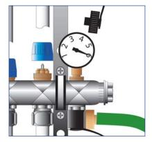
**13.** Allow the pressure to rise to a maximum of 6 bar
