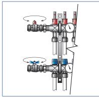
1. Close the isolating ball valves that are connected to the manifold
