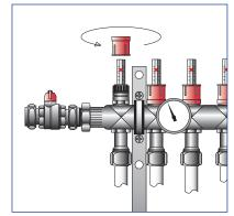
3. Fully open all the flow adjusters on the supply (top) manifold by lifting the red locking collar which may then be used to turn the black collar fully anti-clockwise.
