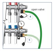
4. Remove the blanking cap from the filling valve on the flow (upper) manifold. Fit the hose connection nozzle (from the *tools and accessories pack*), and connect a suitable hose from the mains water supply. Open the filling valve using key on the blanking cap.
