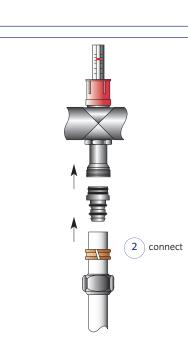
2. Connect the flow pipe to the ports on the upper manifold with the fittings supplied. It is important to make sure that the pipe is securely located. Make sure that the fitting has grasped properly by pulling the pipe.
