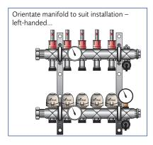
1. Unscrew the manifold-rail mounting clamps, turn the manifold to the correct orientation and re-fit the mounting clamps.
