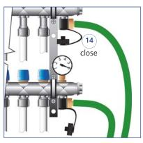
**14**. When the correct pressure is reached, close the filling valve.
