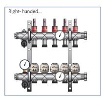
of the pipes. The Supply (flow) manifold must be the rail with the flow gauges.
