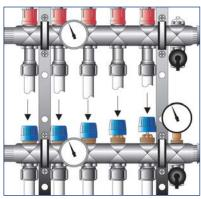
**2.** Isolate all zones by screwing down all the blue protection caps hand tight.
