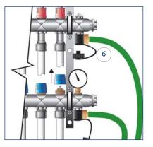
**6**. Fully loosen the protection cap from the first zone to be filled.
