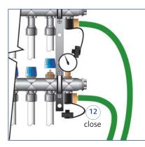
**12.** Close the drain valve on the return (lower) manifold.
