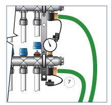
7. Open the tap on the mains water supply and open the drain valve on the return (lower) manifold using key on the blanking cap.
