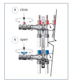
**6**. Shut the flow isolation valve and open the return valve.
