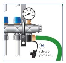
**16.** After testing, reduce the pressure to 1 bar-static by releasing the water from the drain valve on the return(lower) manifold.
