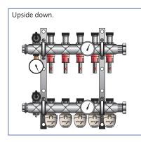
3. Refit the boss on the front of the rail, and the blanking screw on the back. Refit the temperature gauges.
